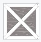
12X Original Strength Building a crate with two diagonal boards on each side increases original strength by nearly 12 times.
